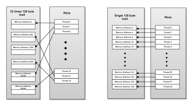
Figure 2: Non coalesced (left) and coalesced (right) memory access.
