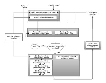
Figure 1: Block diagram of NiftyRegSGD, adding the Random Sampling function to original design of NiftyReg.
