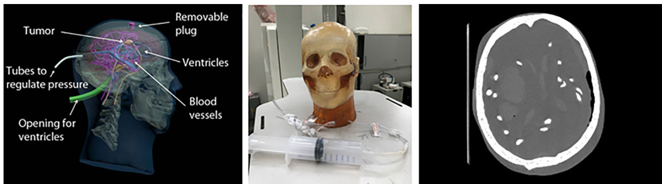
Fig. 2 The computer-aided design model of the anthropomorphic head phantom, the experiment setting and an example slice of CBCT acquisition of the phantom are shown from left to right
